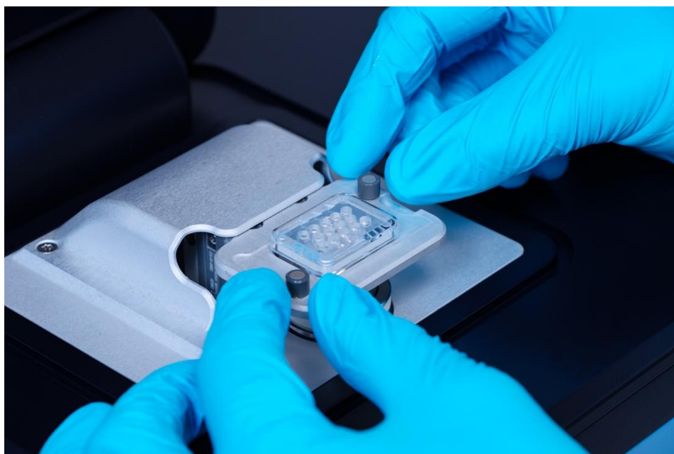
Figure 6: Magnets are placed on the corners of the sample carrier slide to hold it in place.
