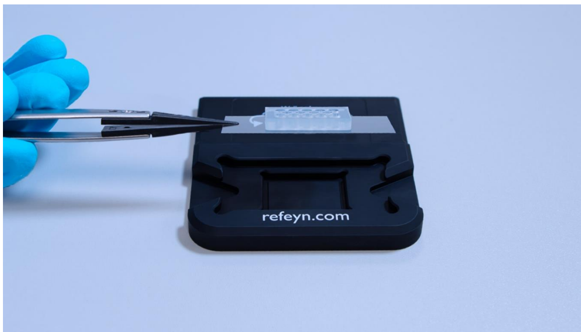
Figure 4: Remove the assembled sample carrier and rotate so the cassette is facing up. Replace in the alignment tool.
