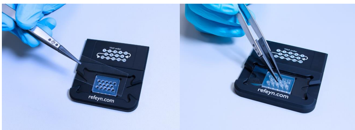
Figure 3: Placing a ready-to-use sample carrier slide on the sample well cassette using the alignment tool
