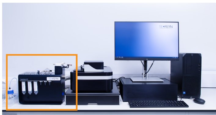
Fig. 1 Refeyn's MassFluidix HC system for rapid dilution via microfluidics. The picture shows a complete mass photometry setup, including MassFluidix HC (left, orange square), the TwoMP mass photometer on an Accurion anti-vibration unit (center) and a computer that controls the instruments (right). Compatible with Refeyn's TwoMP mass photometer, MassFluidix HC enables the analysis of high-concentration samples by mass photometry.
