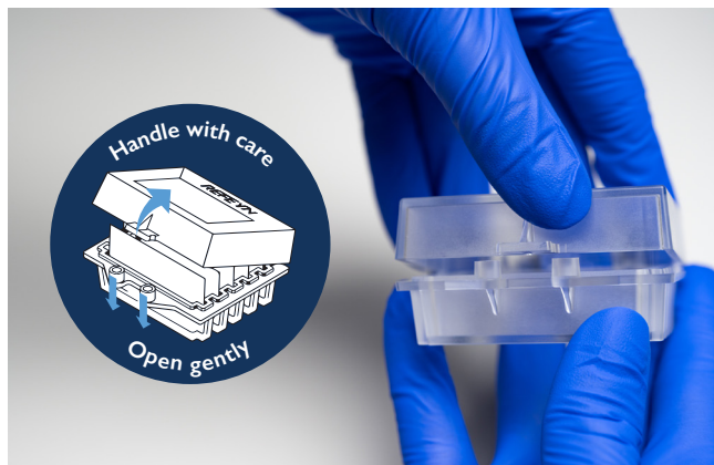
Figure 2. Opening the box. To open the slide box, hold it as shown and gently lift the lid.
